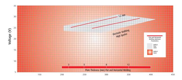
Electrode stick out, contact tip-to-work distance 15 mm for spray. Gas flow rate 18  $\ell$ /min
