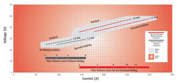
Electrode stick out, contact tip-to-work distance 19-25 mm for spray, 8-13 mm for dip, gas flow rate 15-18  $\ell$ /min
