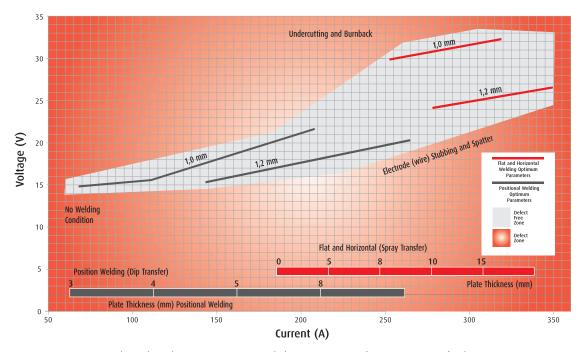
Electrode stick out, contact tip-to-work distance 19-25 mm for spray, 8-13 mm for dip, gas flow rate 15-18  $\ell$ /min
