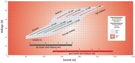
Electrode stick out, contact tip-to-work distance 18 mm for spray, 15 mm for dip, gas flow rate 15 l/min
