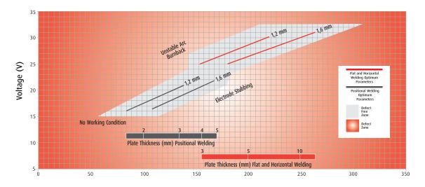
Electrode stick out, contact tip-to-work distance 19-25 mm for spray, 8-13 mm for dip. Gas flow rate 15-18 ℓ/min
