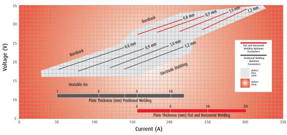
Electrode stick out, contact tip-to-work distance 18 mm for spray, 15 mm for dip, gas flow rate 16 l/min
