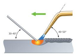
This technique can be used in all welding positions. The method is the same, with the flame following the filler rod, irrespective of the welding position.
