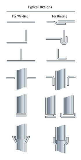
The most common type of joint used for brazing is the lap joint, or the sleeve joint in the case of tubular components. To design a good lap joint, two criteria should be considered:
