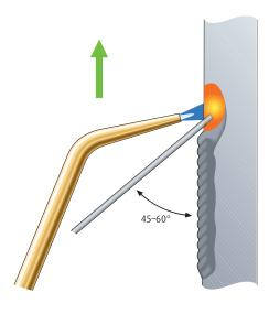
The technique is mainly used for gas welding pipe of all diameters and wall thicknesses up to 6 mm in a single pass, with no edge preparation to the material. This technique was developed to compete with manual metal arc welding and is used mainly on construction sites for welding, heating and ventilating pipe-work.
