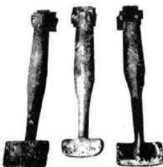
Work railway tampers can be rebuilt by using manual or open arc processes
