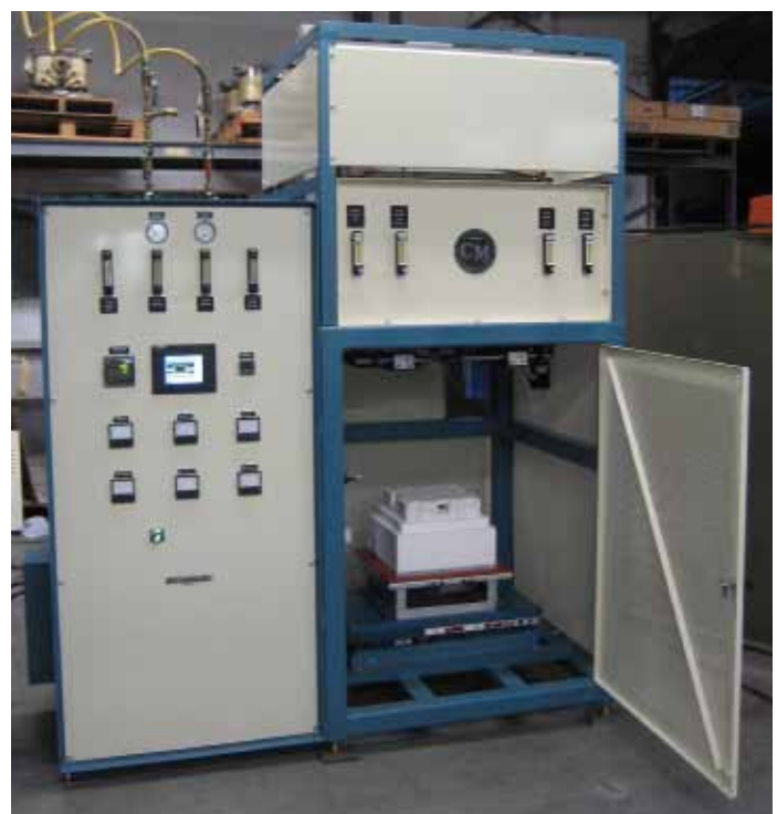
Figure 15: Bell-type box furnace for MIM sintering (courtesy of CM Furnaces Inc.)
