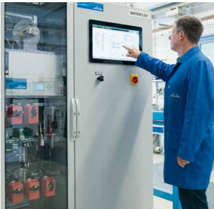
Figure 67: SINTERFLEX™ system with analysing and flow control cabinets; home user screen enlarged in right picture
