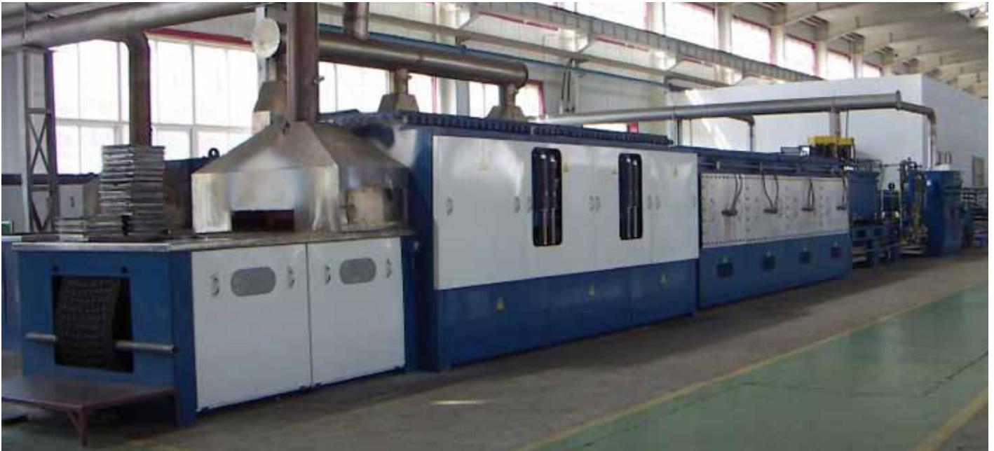
Figure 31: Sintering line with the integrated ADS – Accelerated Delube Station, seen as the second left module in the picture (courtesy of Gasbarre Products Inc.)
