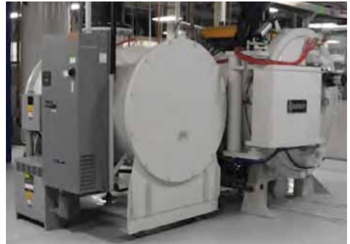
Figure 60: Debinding and sintering furnaces with two bar argon cooling (courtesy of Ipsen)
