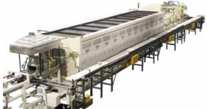
Figure 13: Pusher sintering furnace with molybdenum heating elements for temperatures up to 1600 °C (2910 °F) (courtesy of Abbot Furnace Company)
