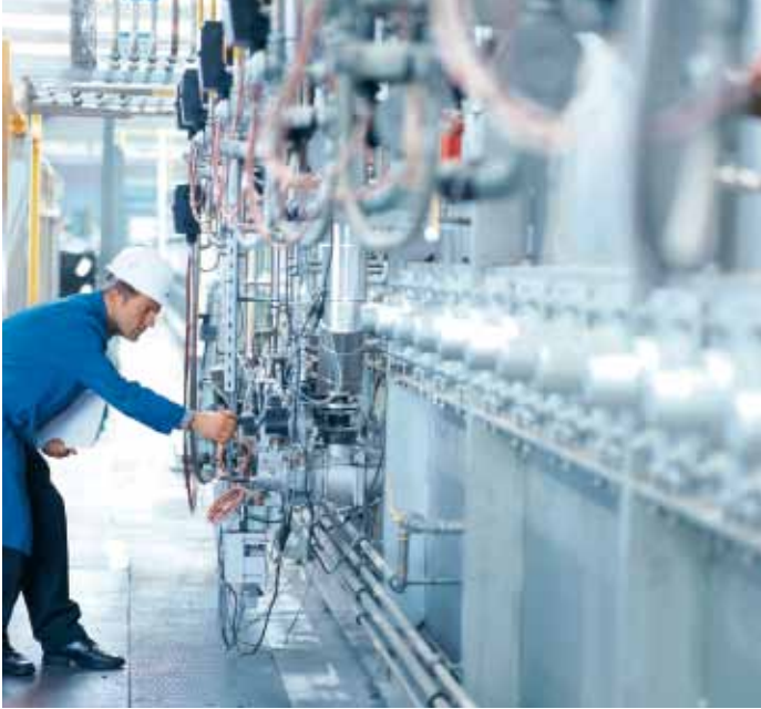
Figure 16: Installation of CARBOJET® effective atmosphere stirring without a fan
