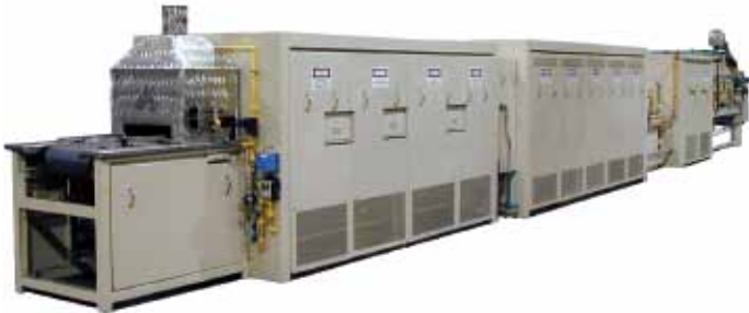
Figure 12: A continuous mesh belt sintering furnace (courtesy of Abbot Furnace Company)
