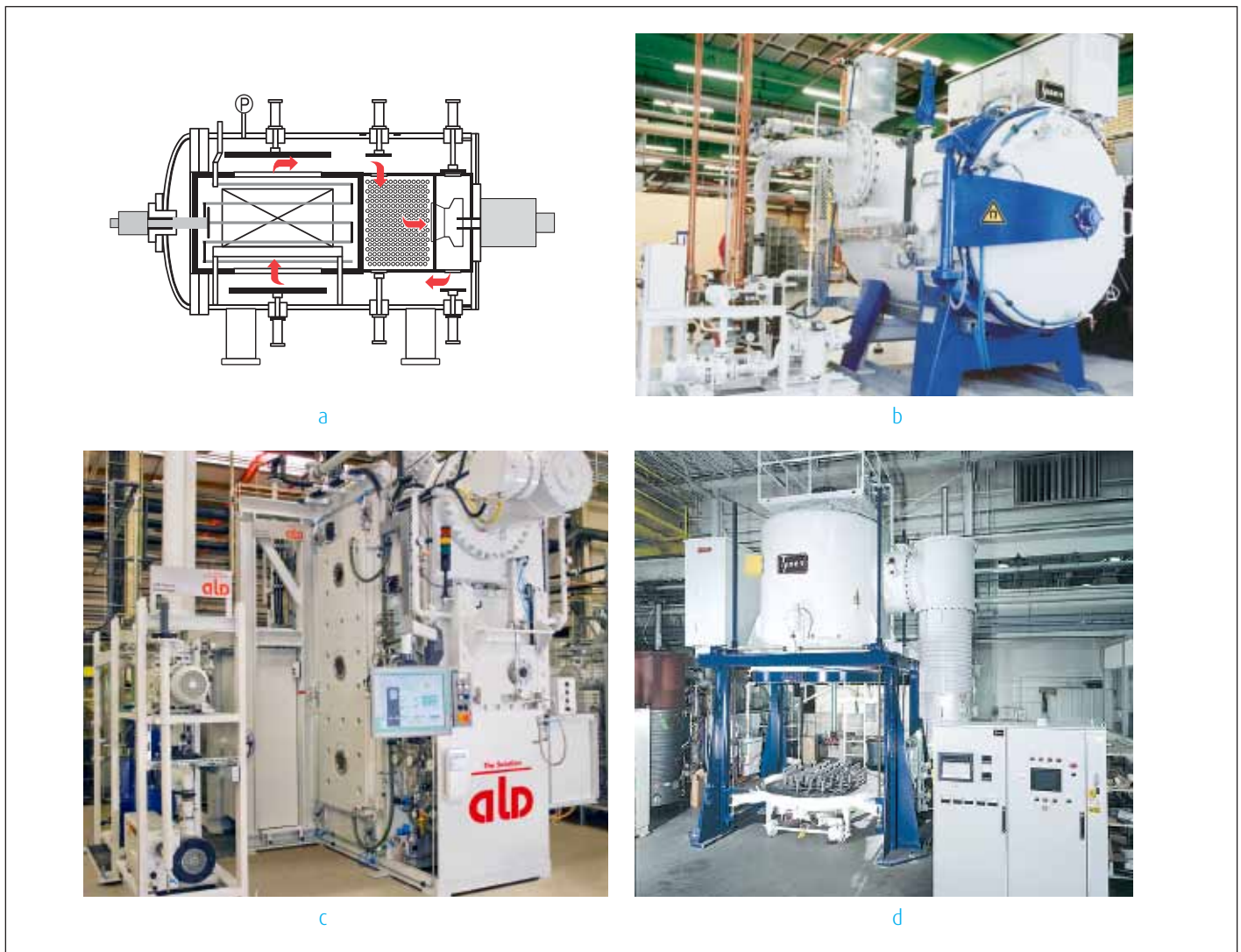
Figure 16: Single-chamber vacuum furnaces: a) Cross section of a single-chamber furnace with integrated high pressure gas cooling, b) single-chamber furnace (Courtesy of Ipsen International GmbH),
