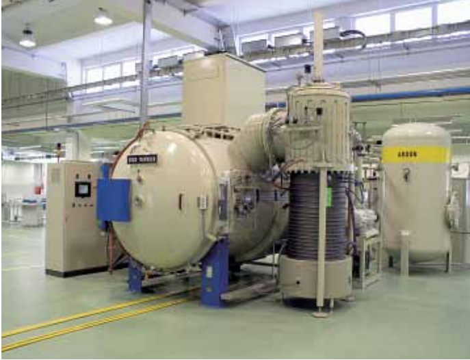
Figure 71: Vacuum furnace with related argon high pressure surge tank, seen on the right (Courtesy of Seco Warwick Corporation).
