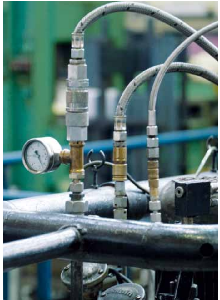
Figure 18: High-pressure nitrogen inlet for the CARBOJET nozzle.
