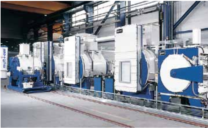
Figure 17: A continuous vacuum furnace hardening line (Courtesy of Ipsen International GmbH).
