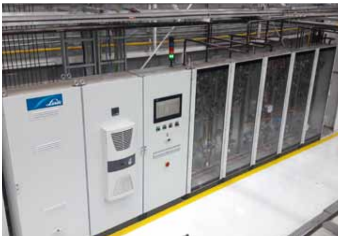
The CARBOFLEX control cabinet: the gas flow adjusts automatically to maintain atmosphere composition within set limits.
