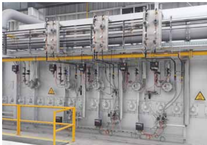
As an essential part of the installation, CARBOCAT® in-situ catalysts are used to produce high-quality endothermic gas.
