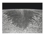
VARIGON He70. Shielding gas for TIG and MIG welding of primarily coarse aluminium. Increased metal penetration and flow with the addition of helium. Enables a higher welding speed.
