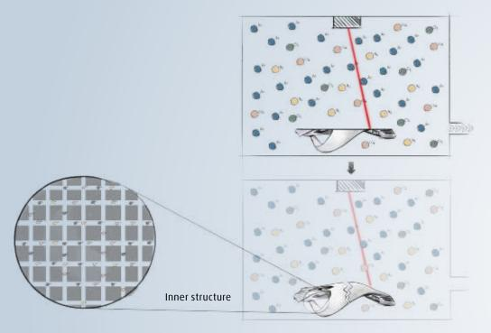
Unwanted gases can enter the AM chamber through insufficient purging, untight connections, or the metal powder itself.
