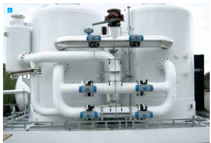
Figure 24: Nitrogen supply methods. a) Storage tank and vaporiser for liquid nitrogen. b) Cryogenic nitrogen production with CRYOSS ® . c) PSA (Pressure Swing Adsorption); ADSOSS ® .
