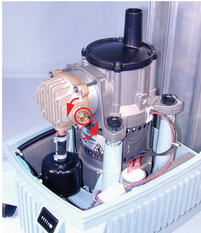
FIGURE AK: REMOVING THE PRESSURE RELIEF VALVE
