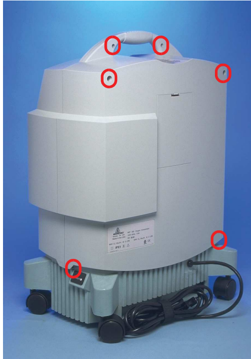
FIGURE AB: REAR CABINET SCREW LOCATIONS
