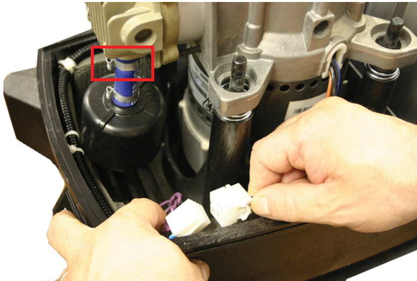
FIGURE AF: DISCONNECTING THE COMPRESSOR ASSEMBLY WIRING HARNESS AND THE LOCATION OF THE ONE-EARED CLAMP
