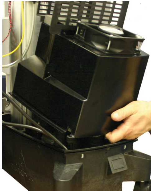
FIGURE AA: REMOVING THE COMPRESSOR COVER (COMPRESSOR COVER SHOWN WITH FAN INSTALLED)
