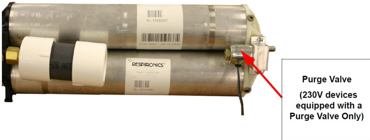
Figure 7-17: PURGE VALVE LOCATION ON SIEVE CANISTER ASSEMBLY
