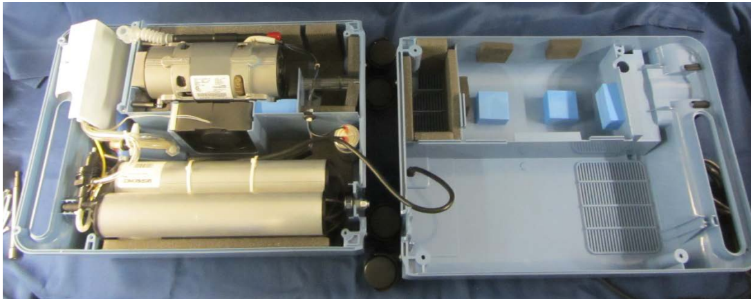
Figure 7-4: EVERFLO REPAIR POSITION
