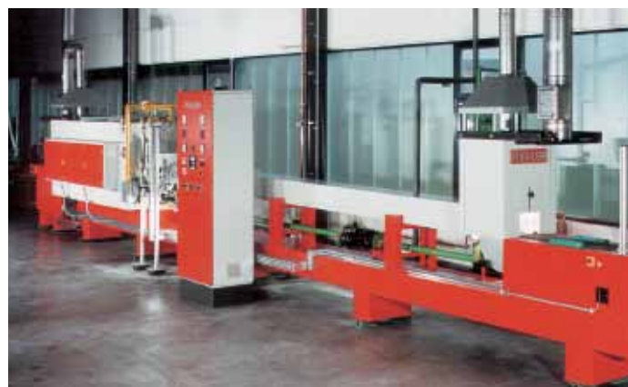
Figure 10: Mesh belt furnace (courtesy of Mahler GmbH)
