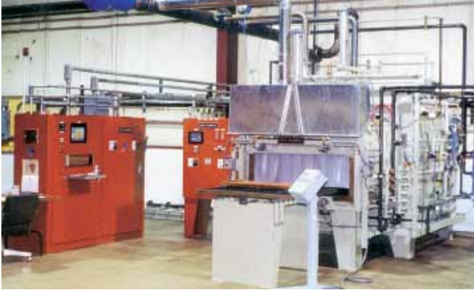
Figure 12: Two-chamber front-loading CuproBraz batch brazing furnace with purging/cooling vestibule and a convection heating chamber (courtesy of SECO/WARWICK Corporation)
