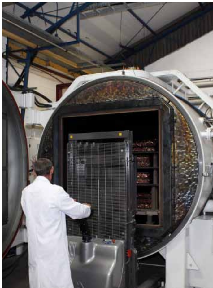
Figure 14: Batch vacuum furnace for brazing (courtesy of Kepston Limited)
