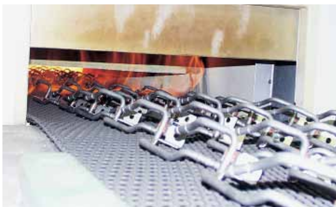
Figure 9: Parts exiting a continuous atmosphere brazing furnace riding on a mesh belt (courtesy of Mahler GmbH)
