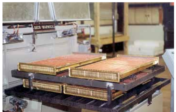
Figure 41: Copper radiators brazed for automotive applications (courtesy of SECO/WARWICK S.A.)
