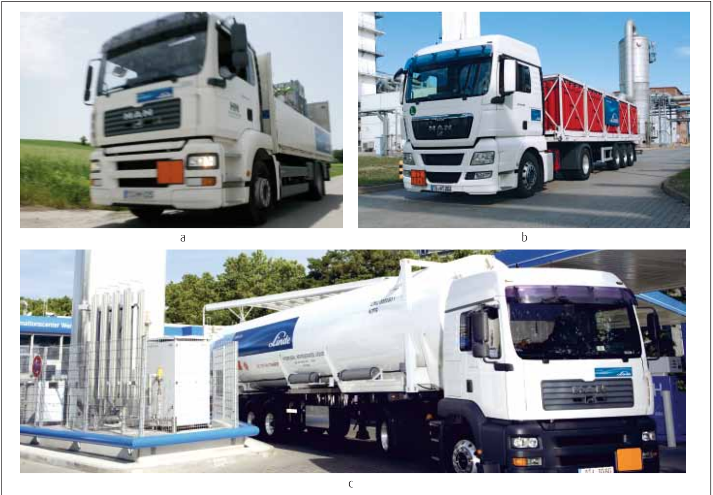
Figure 16: Different supply forms for hydrogen. a) Cylinder bundle with hydrogen, b) Hydrogen tube trailer, c) Liquid hydrogen truck with production facility in the background
