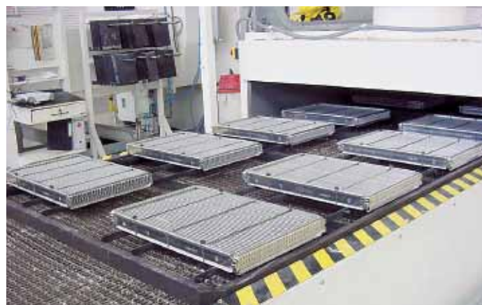
Figure 37: Aluminium heat exchangers entering a CAB furnace (courtesy of SECO/WARWICK S.A.)
