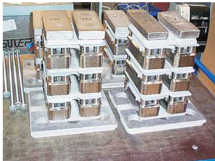
Figure 33: Heat exchangers loaded for brazing [14] (courtesy of Swerim AB). The load to the left marked NA at the top was brazed in argon vacuum. The load to the right marked CA at the top was brazed in argon/hydrogen vacuum
