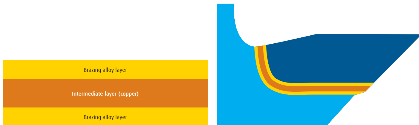
Figure 42: Schematic picture of a trifoil used for joining cemented carbide (courtesy of SAXONIA Technical Materials GmbH)
