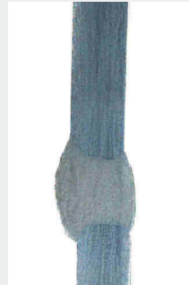
Blech: 3 mm, Spalt: 4 mm, Gas: M21-ArC-18, Draht: 1,9 mm SG3
