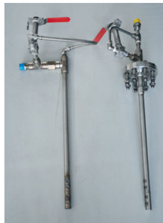
The nozzles shown in the photograph are used for injecting liquid nitrogen into a stream of gas flowing in a pipe to a reactor or other apparatus.
