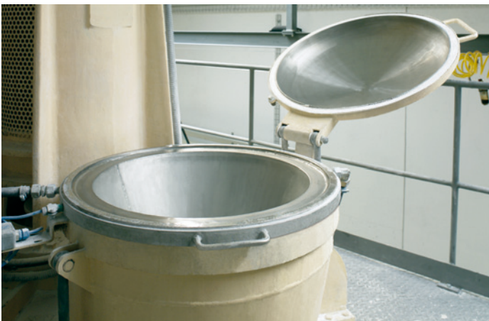
N2LOCK® inert-gas lock integrated into the charging port of a mixer
