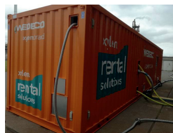
Figure 5. Containerized ozone generator (Xylem Services GmbH)
