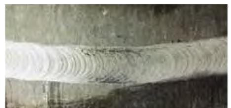
Acier inoxydable stabilisé au titane: protection par Ar/H<sub>2</sub>
