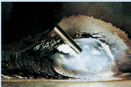
MIG-Schweisnaht an Aluminium
