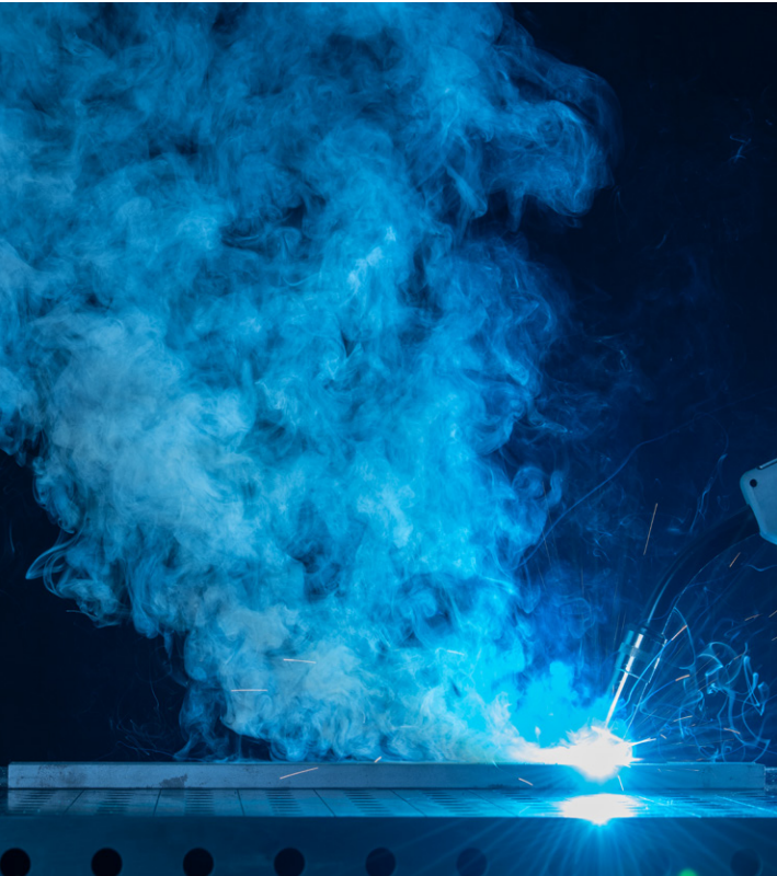
GMAW carbon steel with C25
