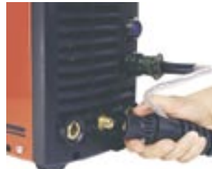
Installing torch cable
