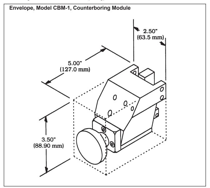
Basic Pipe Sizes: 1" through 2 1/2" pipe all schedules and 3/4" pipe schedules 5S through 40S with the appropriate Clamshell.
