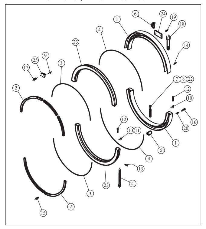
Parts List, Model 642SB, Clamshell Sub-Assembly
