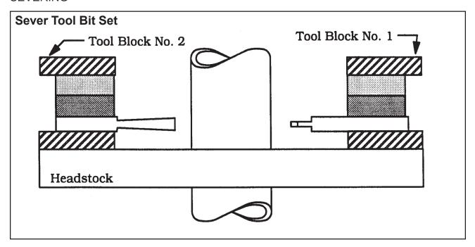
When the Tool Bits sever the pipe, disengage the Feed Pin and let the Headstock rotate 2 to 3 times to clear the chip.
