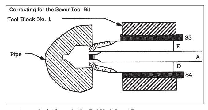
Loosen the Set Screws holding Tool Bits A, D, and E.
