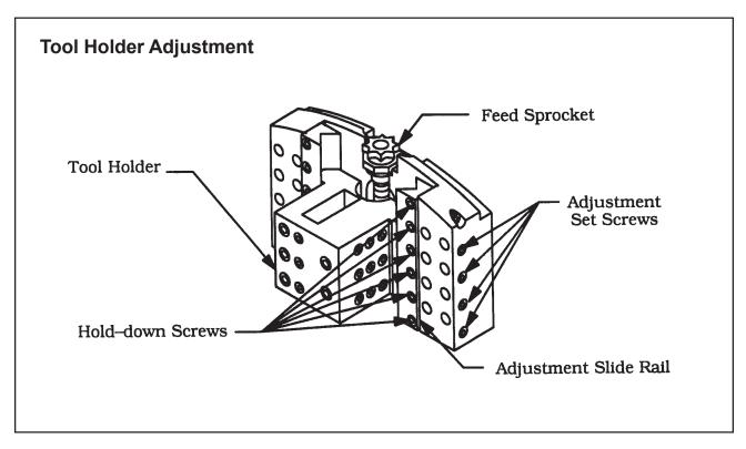
Using the Adjustment Set Screws, apply a light force to the side of the Adjustable Slide Rail so that it is in positive contact with the Tool Holder.
