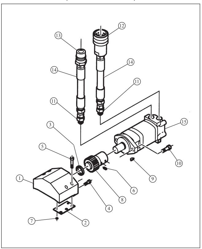
Parts List, Housing and Motor Assembly, Hydraulic (P/N 19-0732 and 56-0044)
