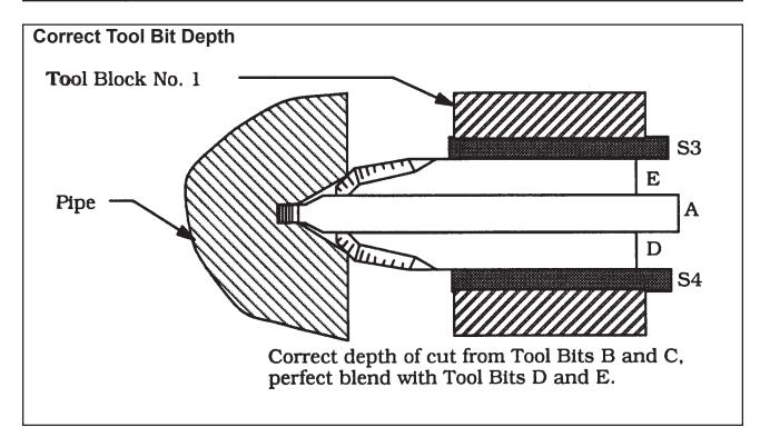
If the cut of Tool Bits B and C is too shallow for a blend with Tool Bits D and E as shown in picture, then proceed on.
