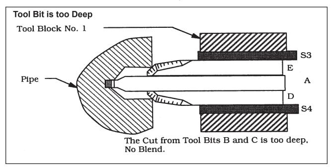
If too deep a cut has been made by Tool Bits B and C as shown, then proceed to "Loosen the Set Screws...."
