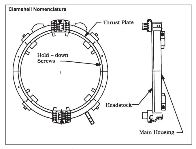
Place the Headstock carefully back into the Housing.
