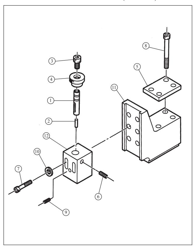
Parts List, Bracket Assembly, Tripper (P/N 47-0447)
