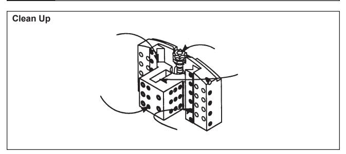
If the Clamshell is operated in such a manner that the Tool Blocks collect debris while cutting, the Tool Blocks and the Feed Screws should be cleaned after each cutting operation.
