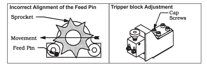
If the Feed Pin to Sprocket engagement is as shown in 'Incorrect alignment of the Feed Pin', then it will be necessary to loosen the four (4) Cap Screws on the Tripper Bracket, so that it may be adjusted to the proper gap [.020" to .030" (.51 mm to .76 mm)] required for proper engagement.
