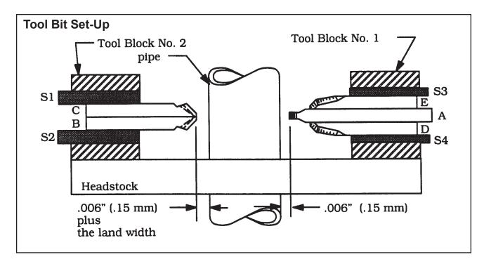
While rotating the Headstock, visually determine the point on the surface where Tool Bit A comes closest to the pipe.
