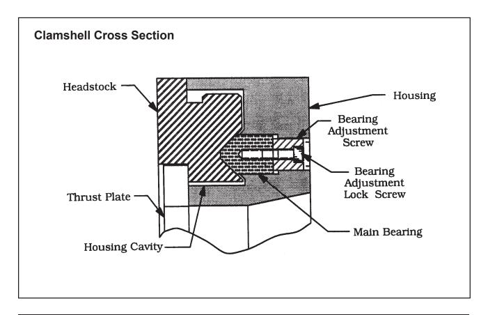
Turn in Bearing Adjustment Screws (1, 6, 11, 16, 21, and 26) so that they are snugged tightly.
