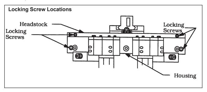
Rotate the Headstock until the split-lines of the Headstock match the split-lines of the Housing.
