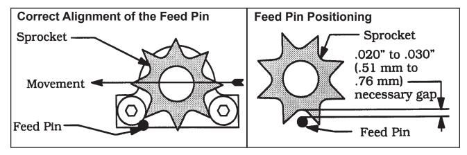
See the above pictures for the correct Feed Pin to Sprocket engagement.
