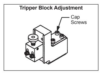
If the Feed Pin to Sprocket engagement is as shown (in picture above), then it will be necessary to loosen the four (4) Cap Screws on the Trippper Bracket, so that it may be adjusted to the proper gap (.020" to .030")(.51mm to .76 mm) required for proper engagement.
