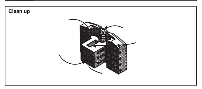
If the Clamshell is operated in such a manner that the Tool Blocks collect debris while cutting, the Tool Blocks and the Feed Screw should be cleaned after each cutting operation.
