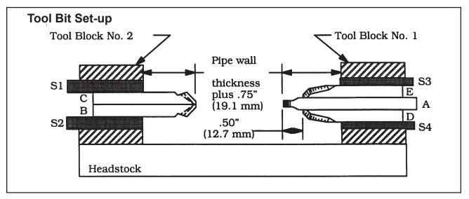
Position the Spacers flush with the inside face of the Tool Holder.
