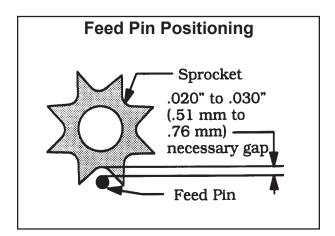
The Feed Pin must not strike the Sprocket Tooth straight on.
