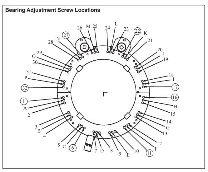
Relax Bearing Adjustment Set Screws (1, 6, 11, 16, 17, 22, 27 and 32) and resnug them so that all of the Bearing Adjustment Set Screws are evenly loaded against the Bearing.
