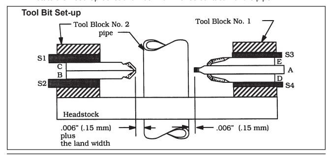
Back the Tool Holder away from the pipe about 1/4 of a revolution. (Approximately .008")(.20 mm).
