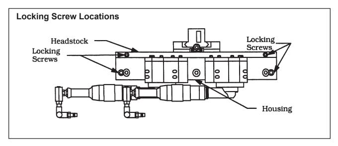
Rotate the Headstock by hand until the split-lines of the Headstock match the split-line of the Housing.
