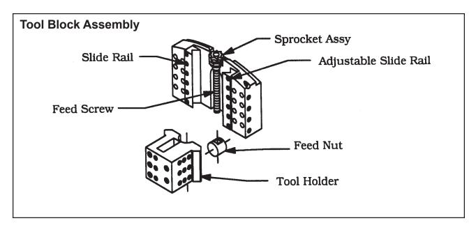
Adjust the adjustable Slide Rail to provide a firm, but not excessive rotational pressure on the sprocket.
