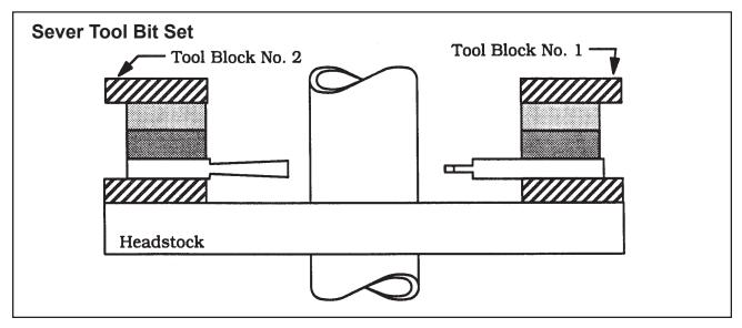
When the Tool Bits sever the pipe, disengage the Feed Pin and let the Headstock rotate 2 to 3 times to clear the chip.
