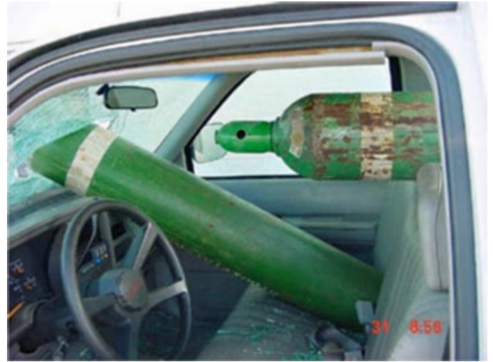
Damage from inappropriately stored and unrestrained cylinders in a vehicle, which stopped suddenly. Please note: Image is for illustrative purposes only. Cylinder colours do not comply with Australian Standards.
